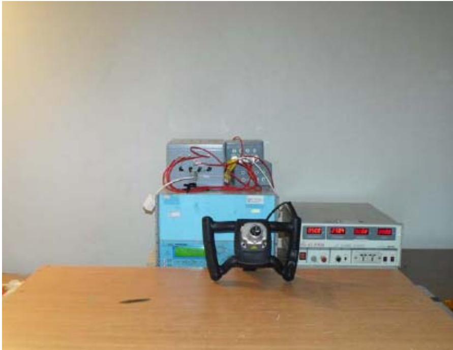
Figure 6 Harmonics & Flicker & Surge & DIPS test setup
