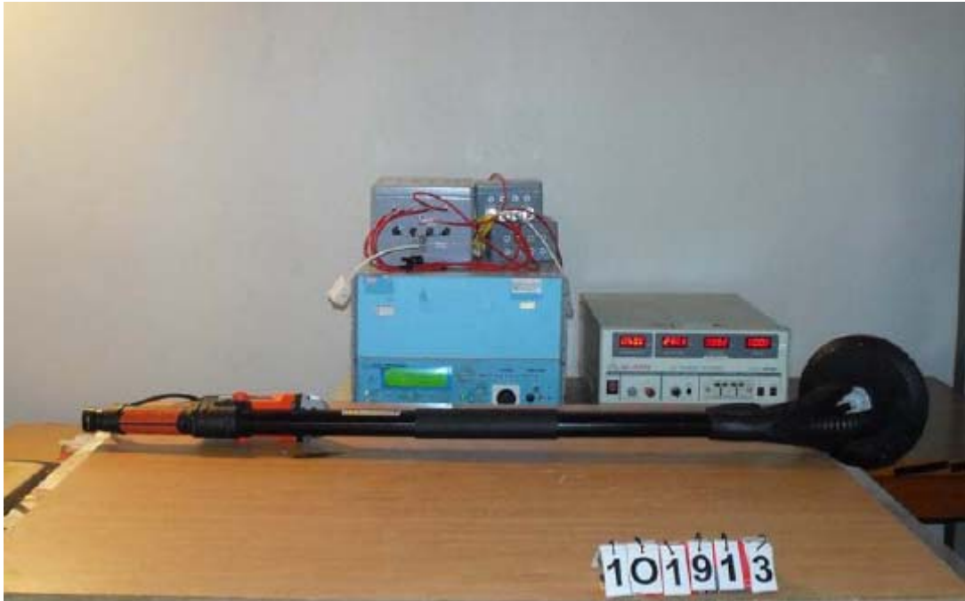
Figure 5 Harmonics & Flicker & Surge & DIPS test setup
