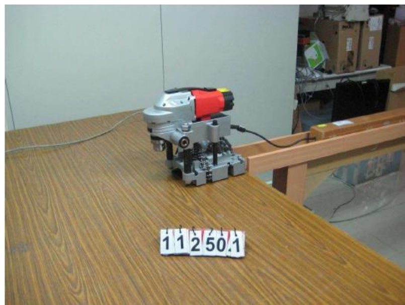
Figure 4 Disturbance power test setup
