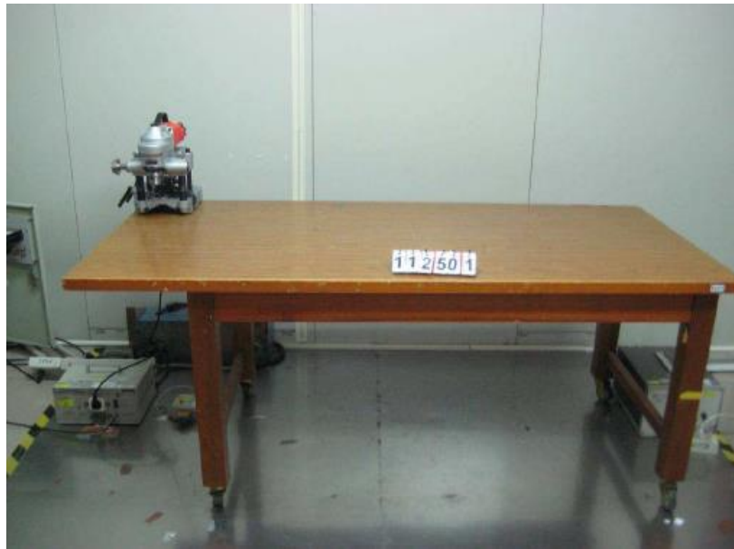
Figure 3 Conducted Emission test setup
