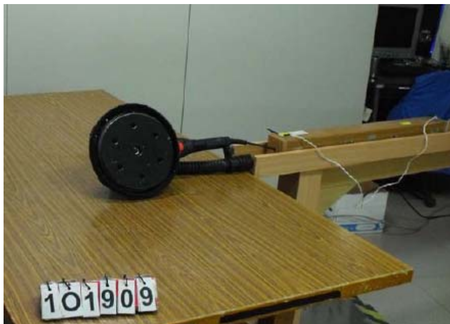
Figure 4 Disturbance power test setup
