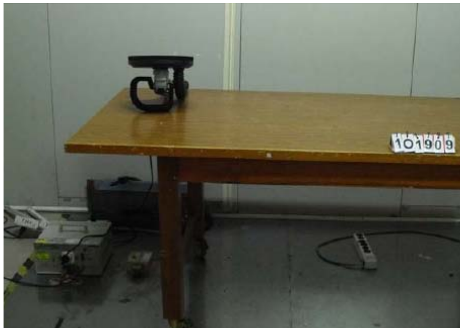
Figure 3 Conducted Emission test setup
