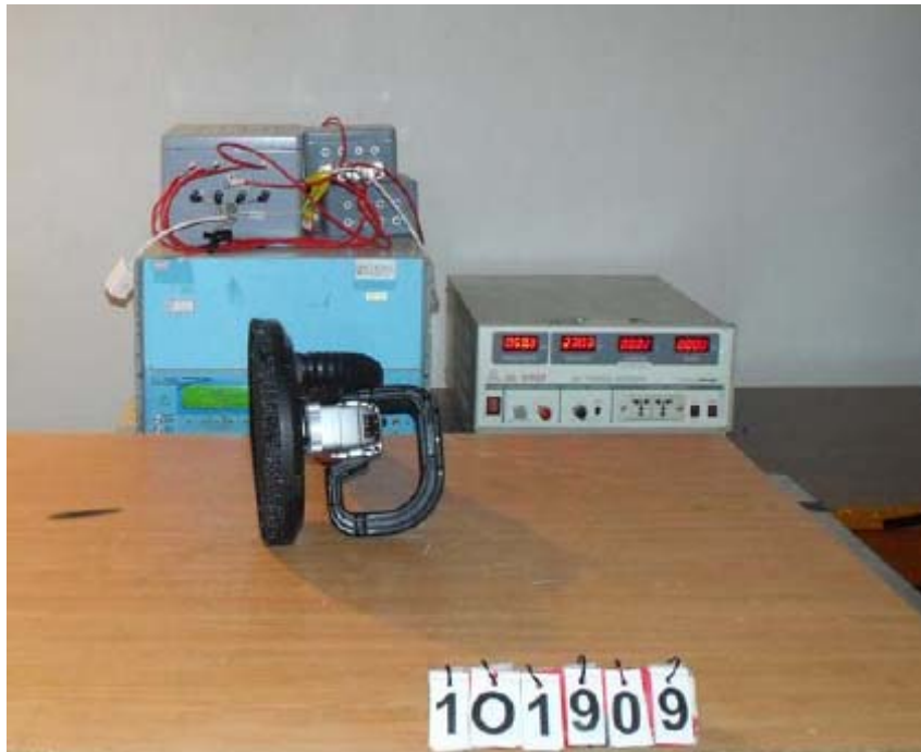
Figure 5 Harmonics & Flicker & Surge & DIPS test setup
