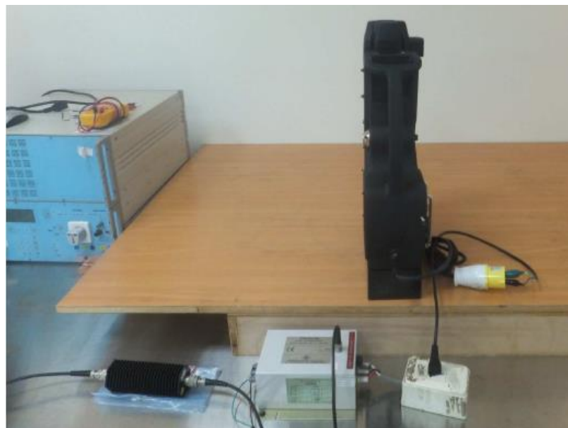
Figure 8 CS test setup
