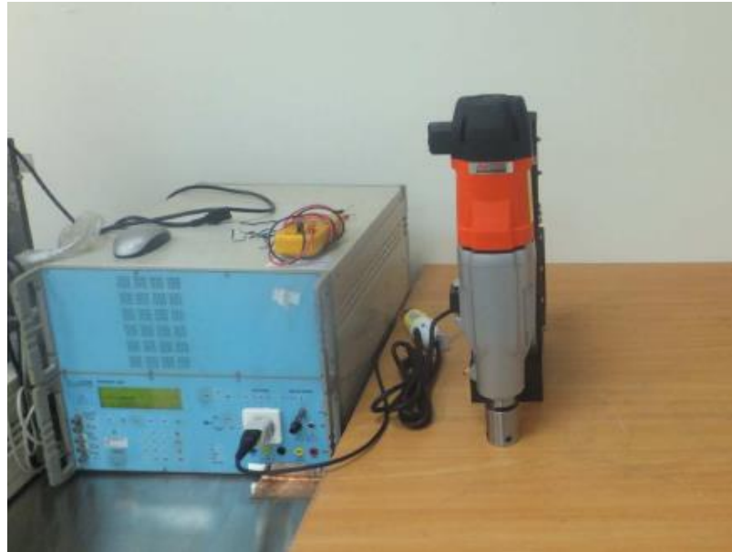
Figure 5 Harmonics & Flicker & Surge & DIPS test setup
