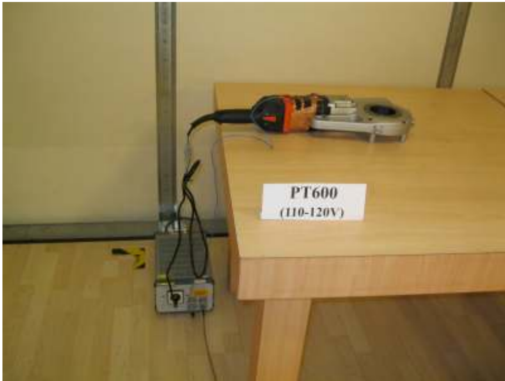
Picture 1: Test setup for Conducted Emission, PT600 (AC 110-120V)
