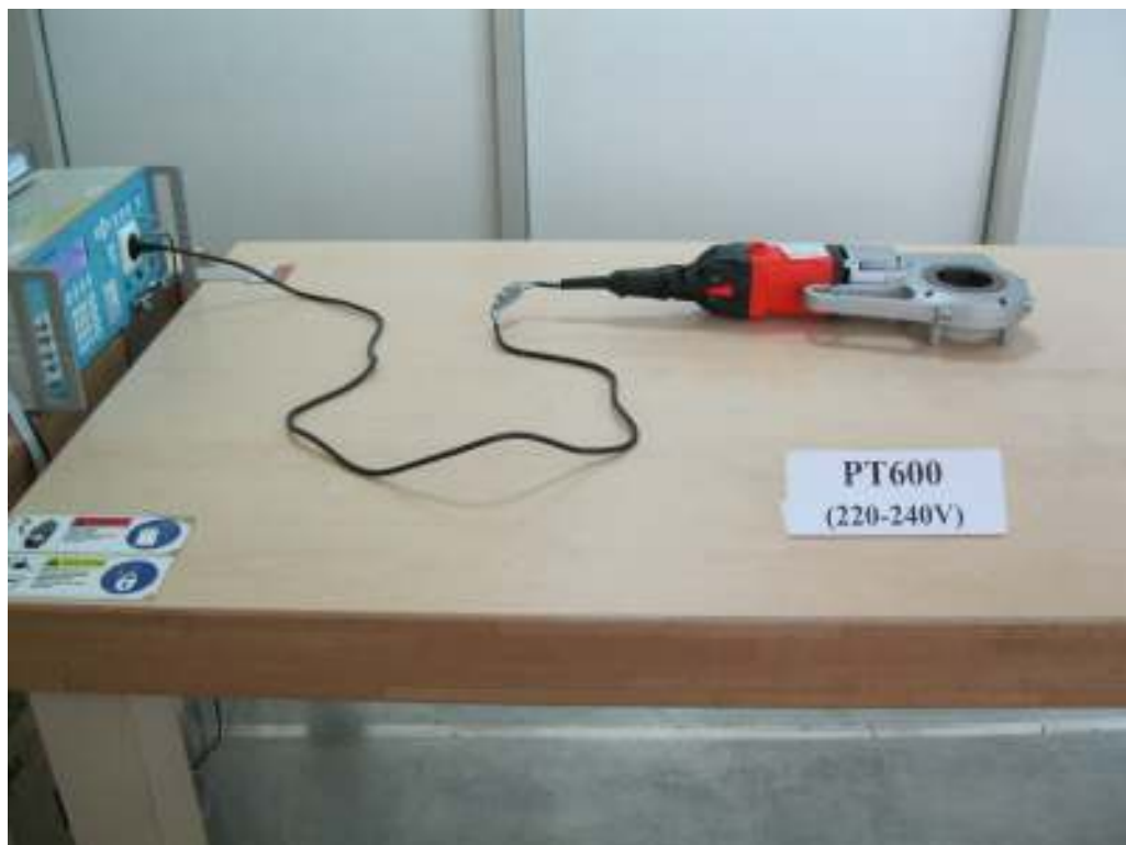
Picture 10: Test setup for Voltage Dips and Interruptions, PT600 (AC 220-240V)
