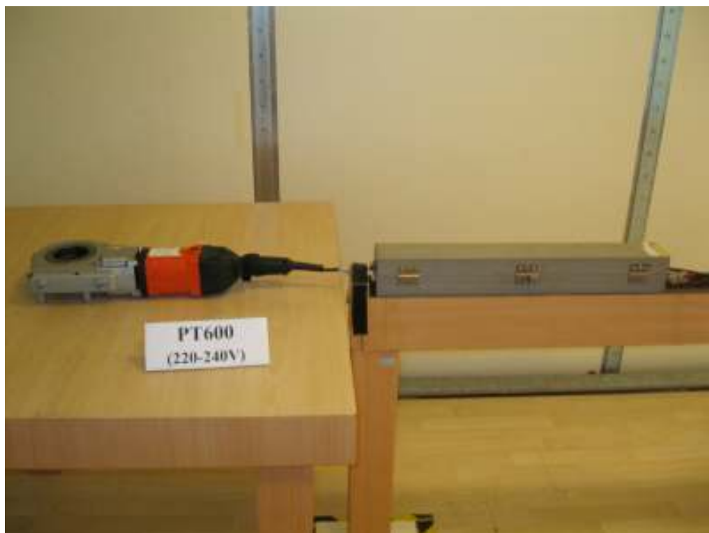
Picture 4: Test setup for Disturbance Power, PT600 (AC 220-240V)
