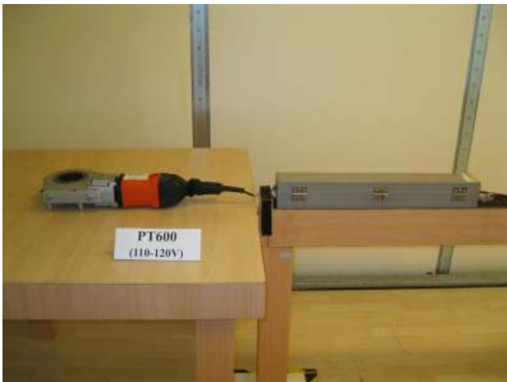
Picture 2: Test setup for Disturbance Power, PT600 (AC 110-120V)
