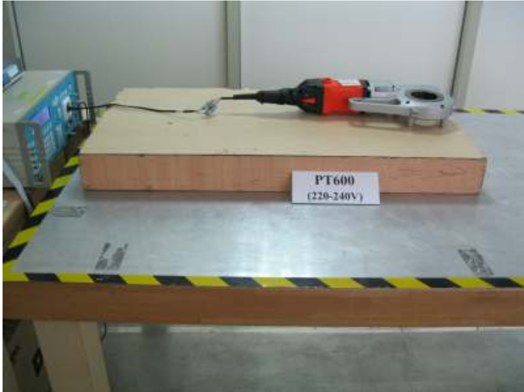
Picture 7: Test setup for Electrical Fast Transient, PT600 (AC 220-240V)
