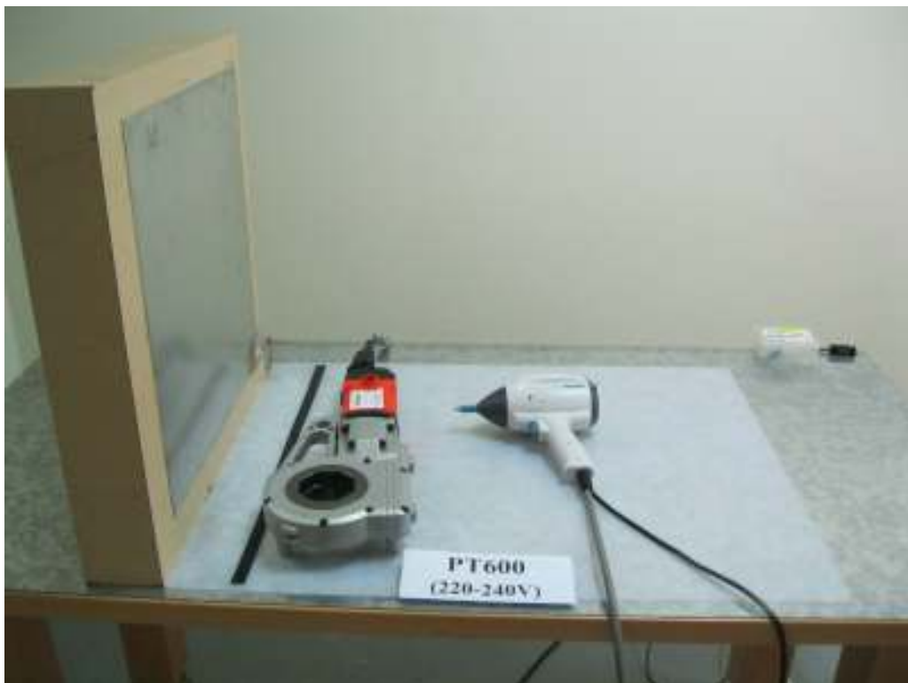
Picture 6: Test setup for Electrostatic Discharge, PT600 (AC 220-240V)
