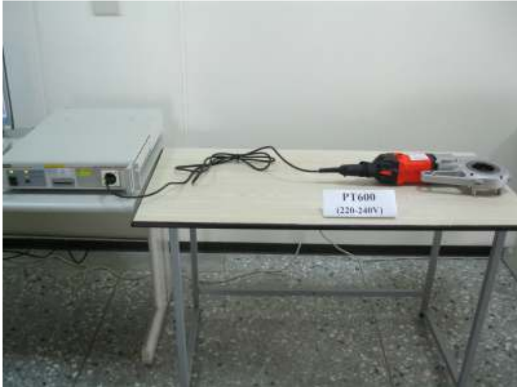
Picture 5: Test setup for Harmonics and Flickers, PT600 (AC 220-240V)
