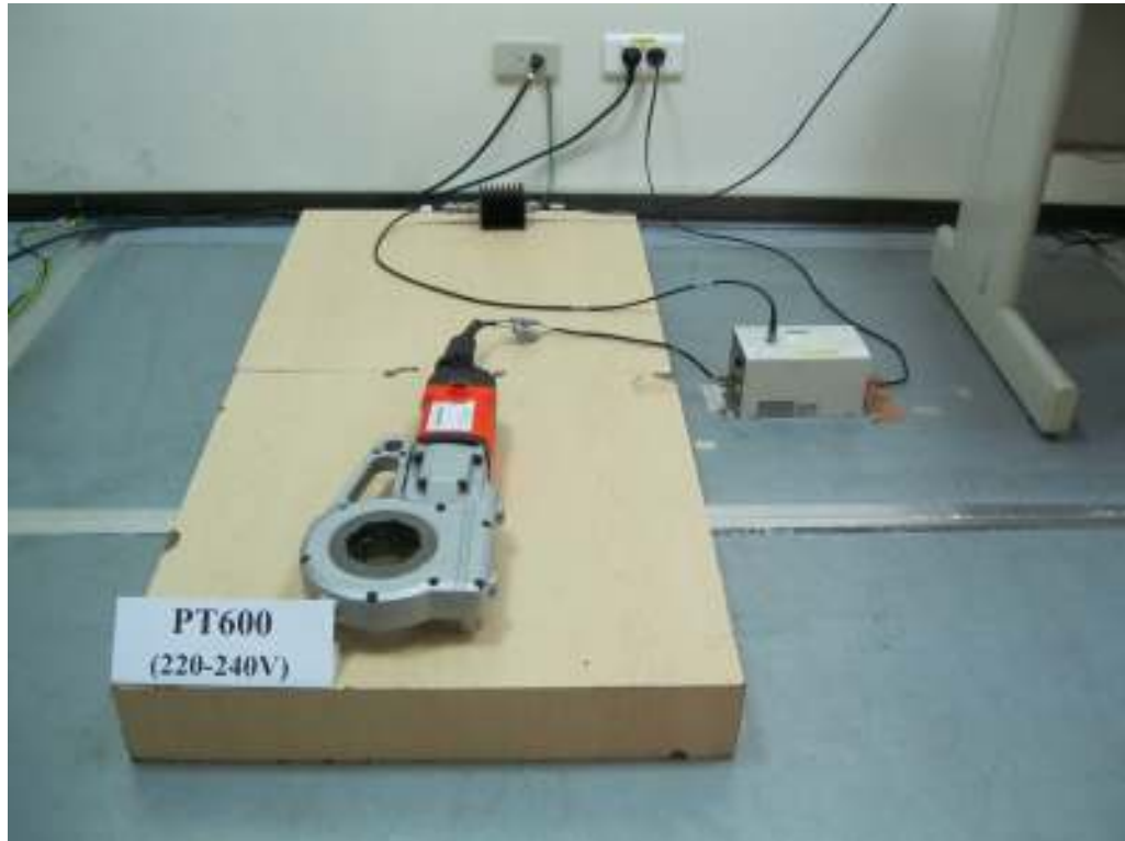
Picture 9: Test setup for Conducted Susceptibility, PT600 (AC 220-240V)
