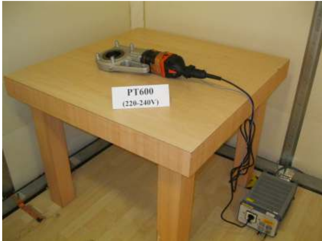
Picture 3: Test setup for Conducted Emission, PT600 (AC 220-240V)
