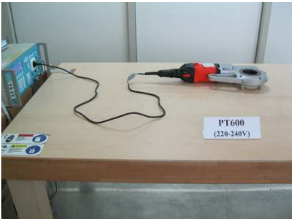
Picture 8: Test setup for Surge, PT600 (AC 220-240V)
