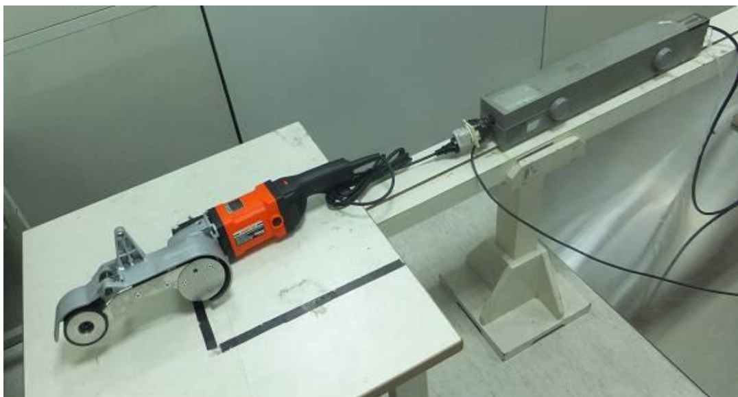
Figure 5 Disturbance power test setup
