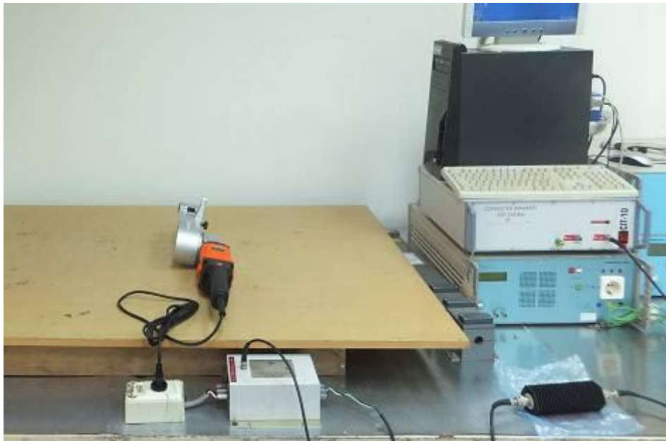
Figure 9 RF Conducted immunity test setup
