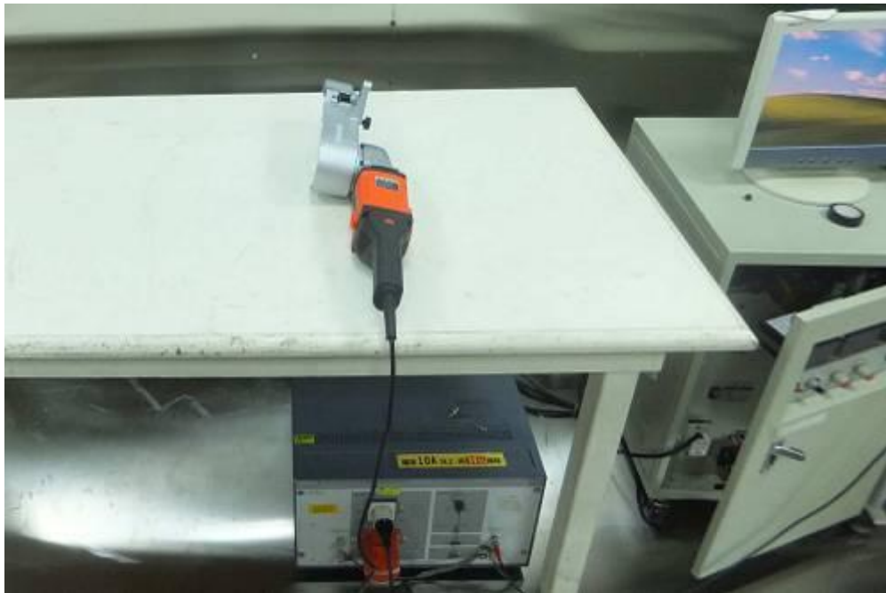
Figure 4 Conducted Emission test setup
