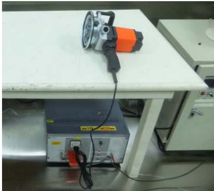
Figure 2 Conducted Emission test setup
