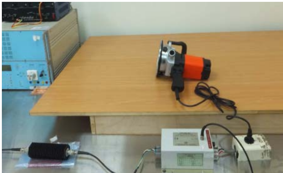
Figure 7 CS test setup
