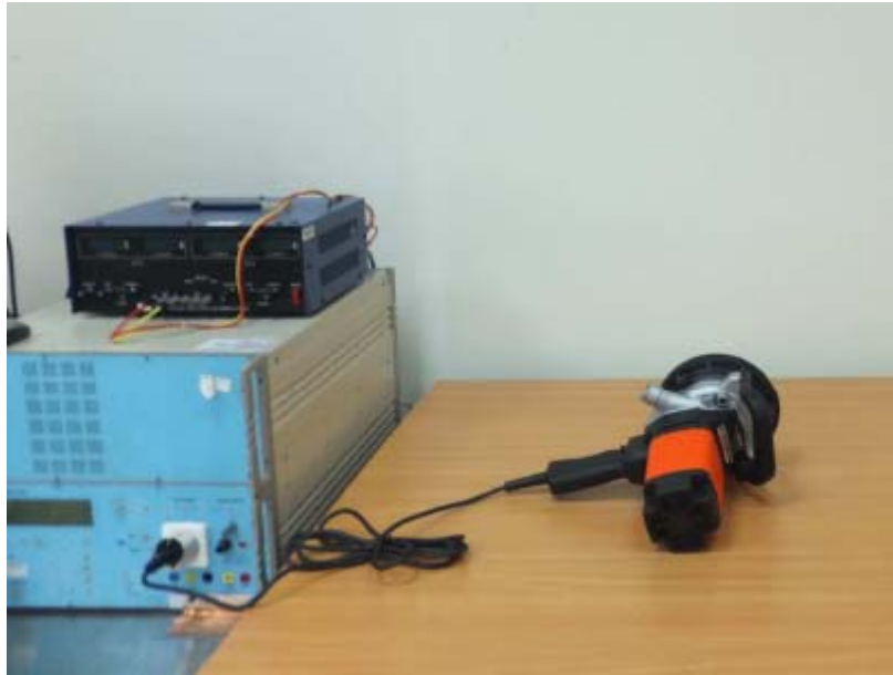
Figure 4 Harmonics & Flicker & Surge & DIPS test setup
