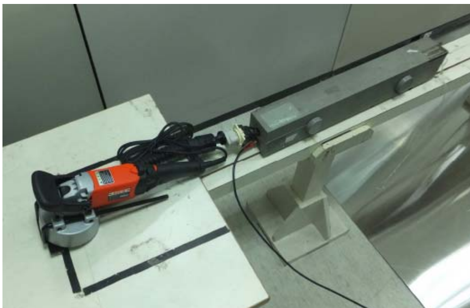
Figure 5 Disturbance power test setup
