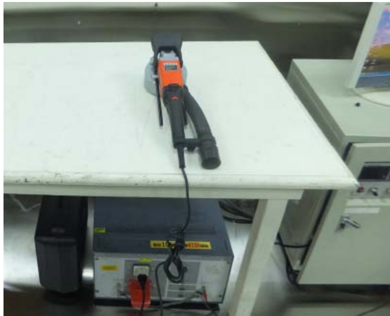
Figure 4 Conducted Emission test setup
