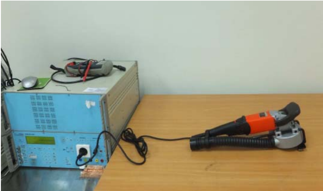
Figure 6 Harmonics & Flicker & Surge & DIPS test setup
