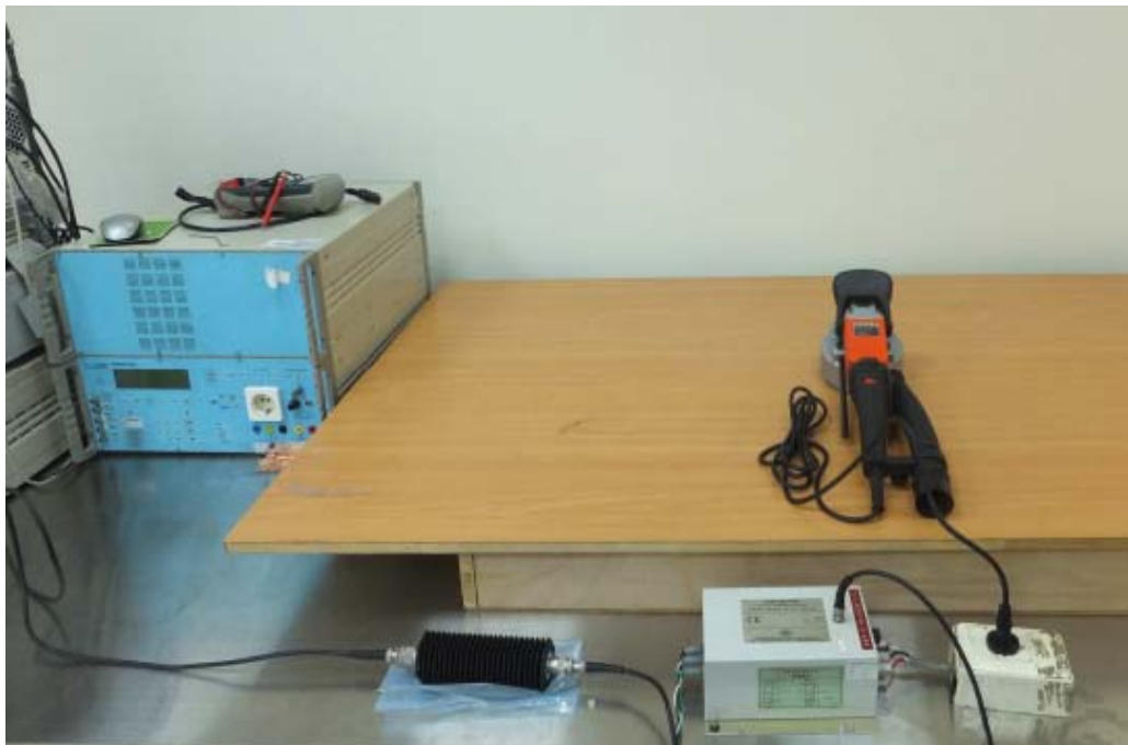
Figure 9 Conducted RF disturbances test setup
