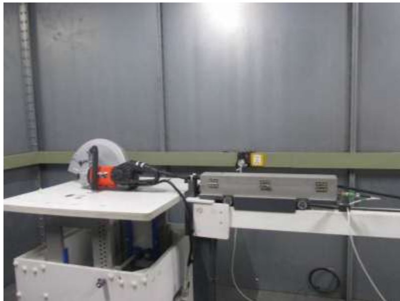
Figure 3 Disturbance power test setup
