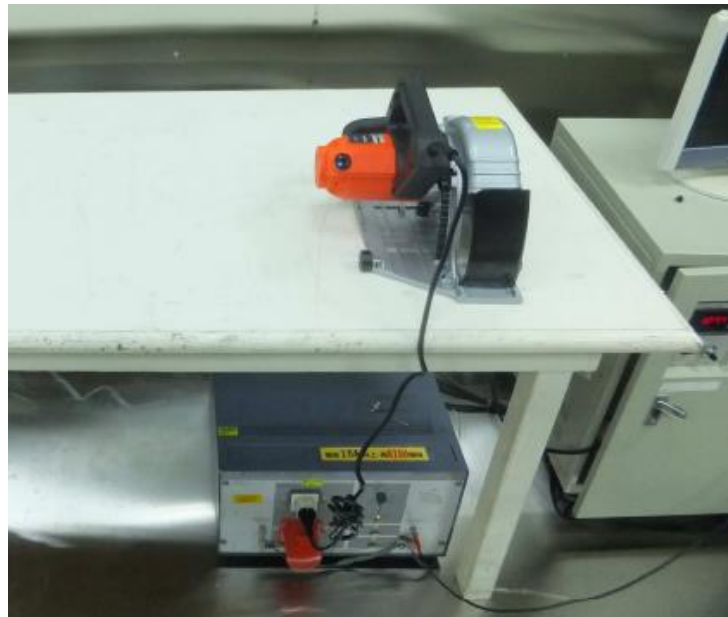
Figure 4 Conducted Emission test setup
