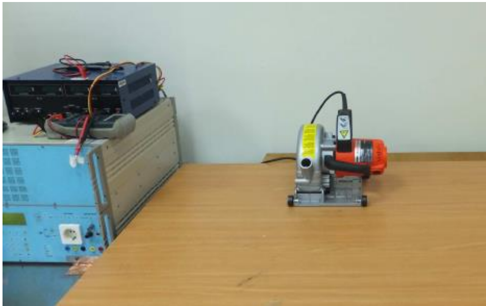
Figure 6 Harmonics & Flicker & Surge & DIPS test setup
