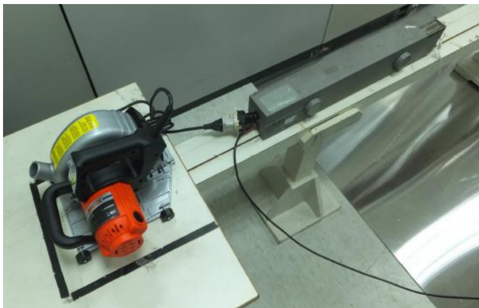
Figure 5 Disturbance power test setup
