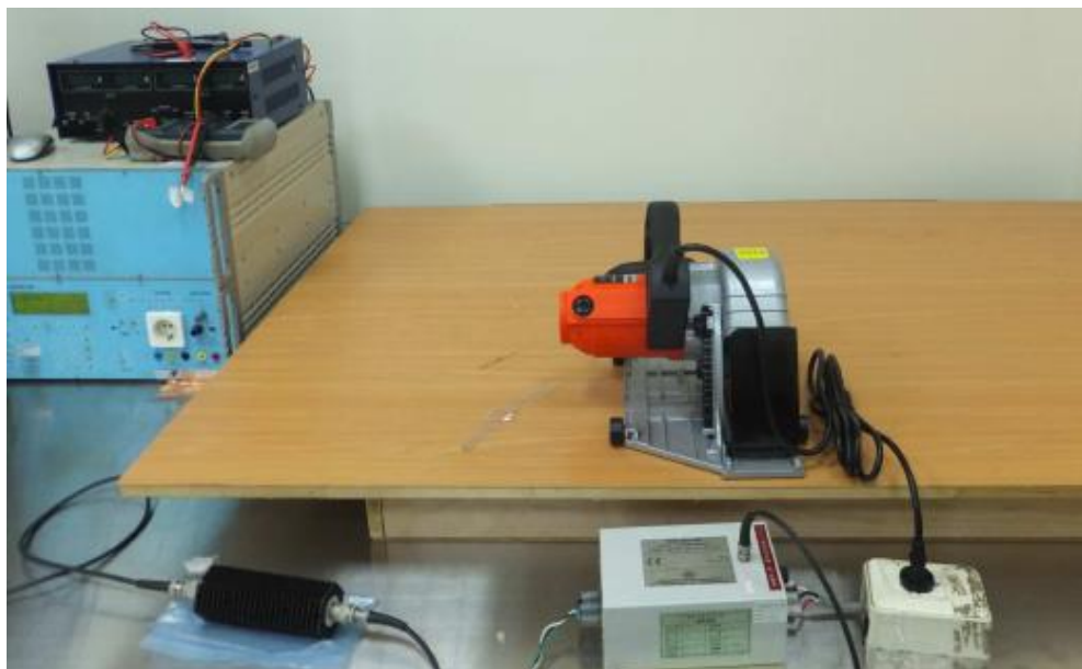
Figure 9 RF Conducted immunity test setup
