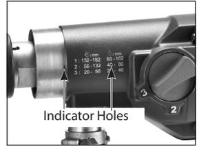
**CAUTION: There are two small holes on the top of the gearcase. If either of these holes leaks water, it indicates that the water seals are worn out. Replace them immediately.**
