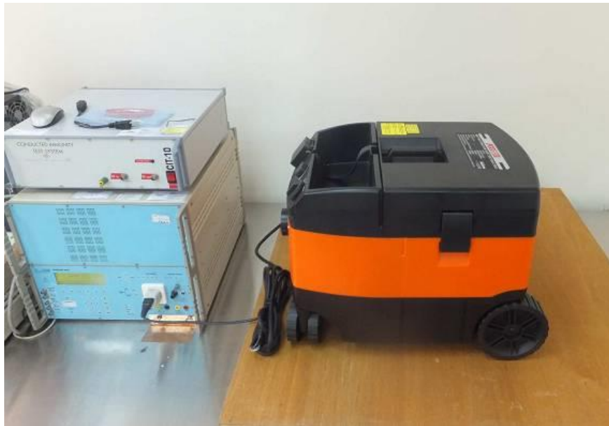
Figure 8 EFT & Surge & DIPS test setup
