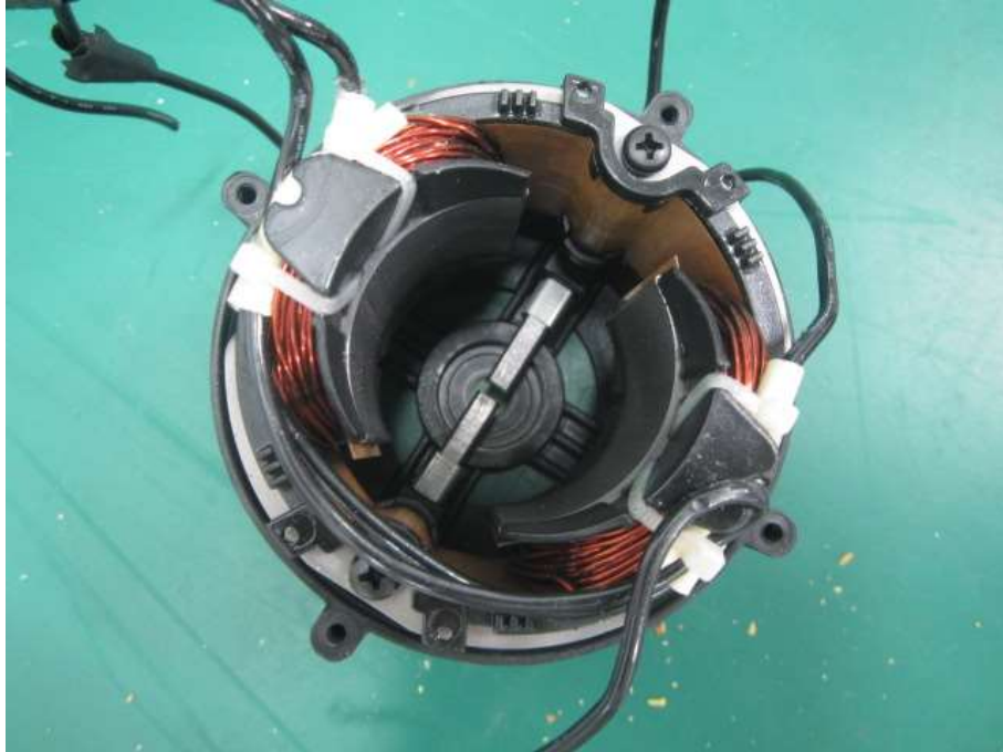
Pic.23 Stator windings
