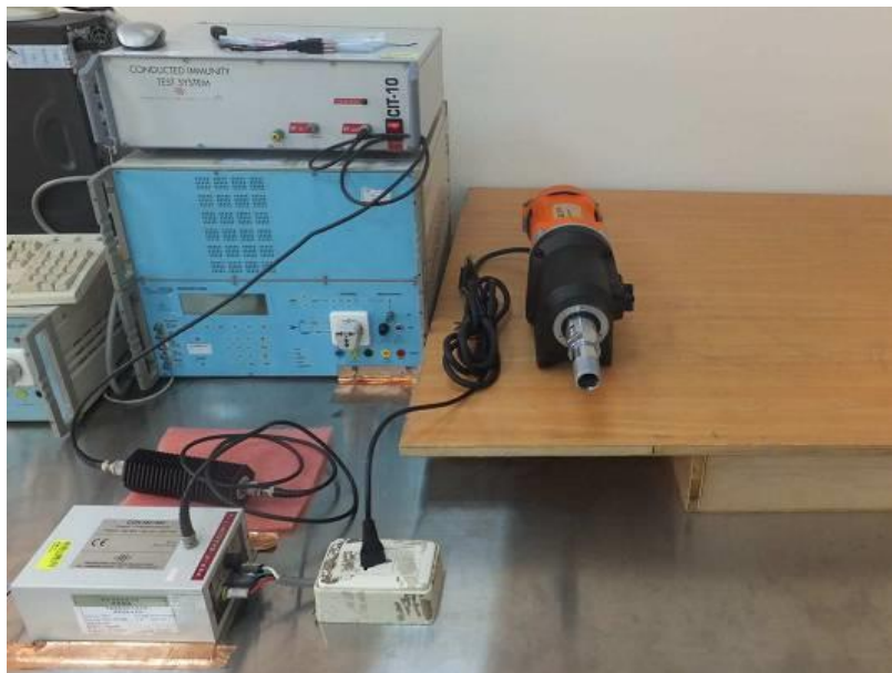
Figure 9 RF Conducted immunity test setup
