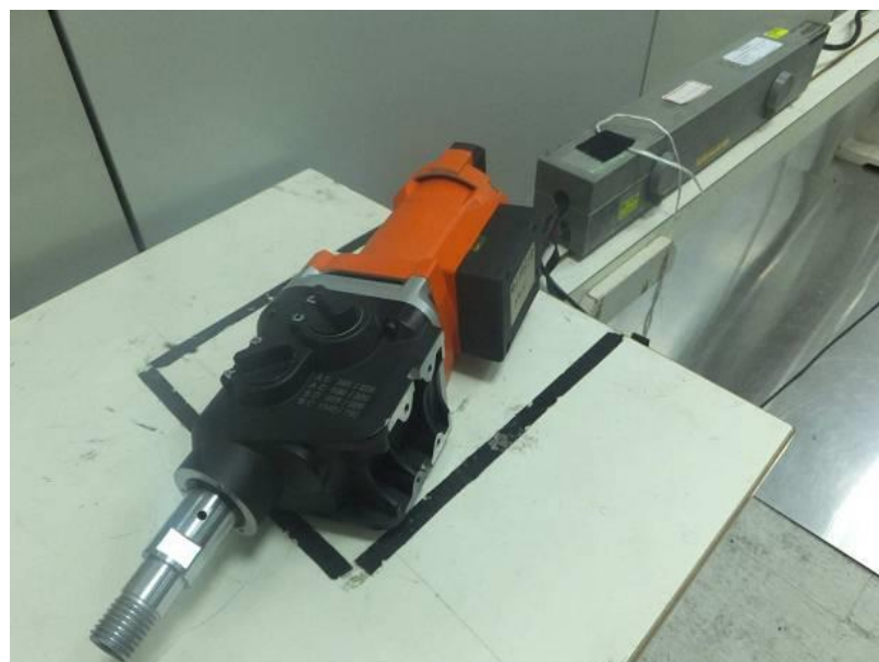
Figure 5 Disturbance power test setup
