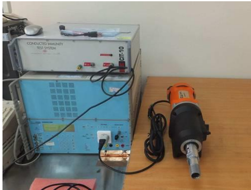
Figure 8 EFT & Surge & DIPS test setup
