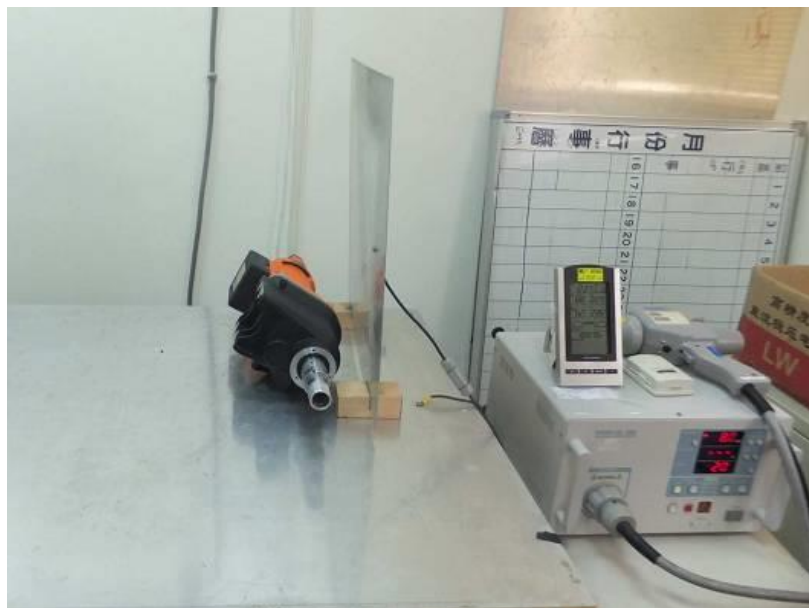
Figure 7 ESD test setup
