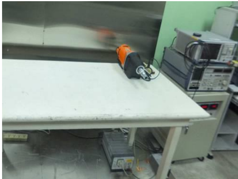
Figure 4 Conducted Emission test setup
