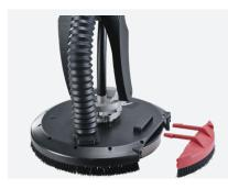
Half-Moon Door With the half-moon door temporarily removed, the edge cutout in the dust skirt allows sanding right up to the edge in corners.
