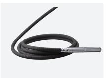
No Driveshaft in the Hose This design gives much higher vibrating efficiency than drive cable type vibrators, since the hose only carries the electrical wires, meaning that there are no friction problems and power losses from a drive cable.
