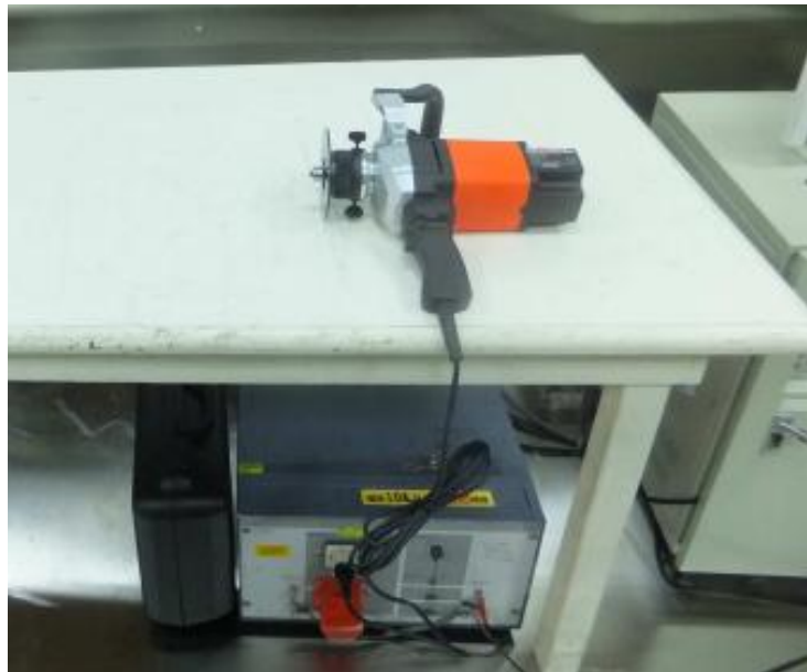
Figure 3 Conducted Emission test setup
