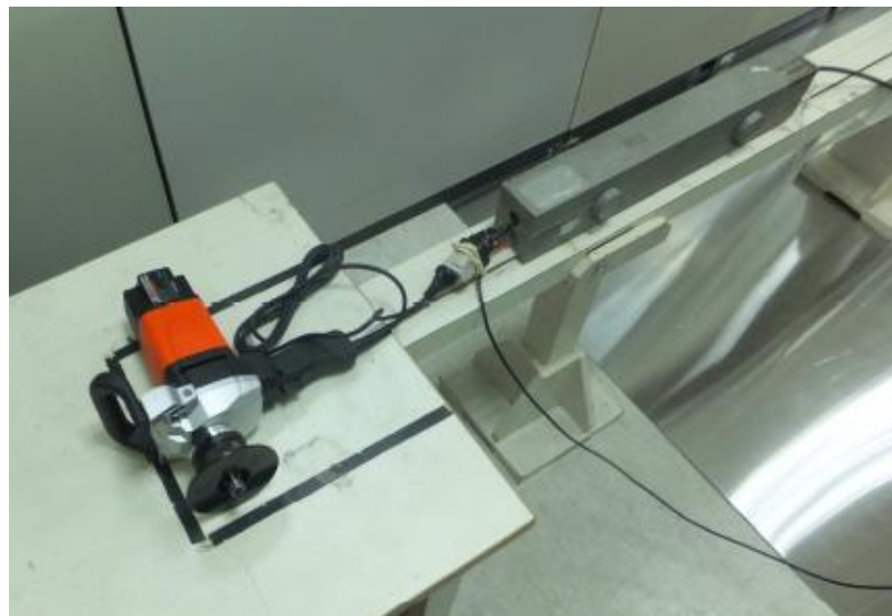
Figure 4 Disturbance power test setup
