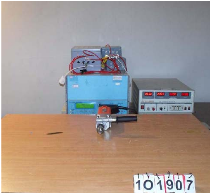
Figure 4 Harmonics & Flicker & Surge & DIPS test setup
