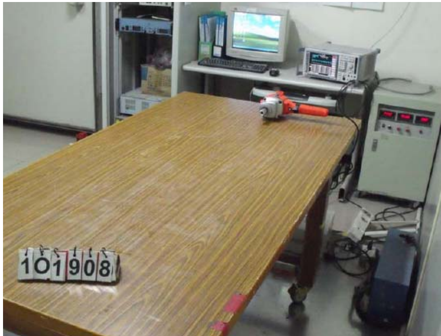
Figure 2 Conducted Emission test setup
