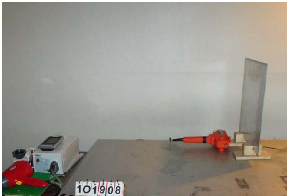
Figure 5 ESD test setup
