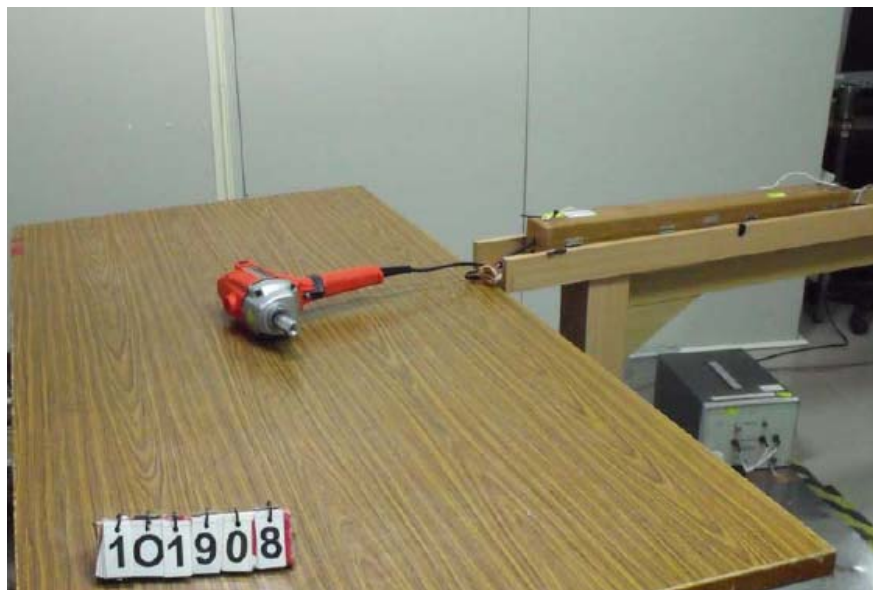
Figure 3 Disturbance power test setup
