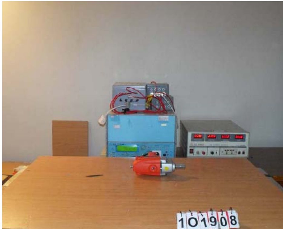
Figure 4 Harmonics & Flicker & Surge & DIPS test setup
