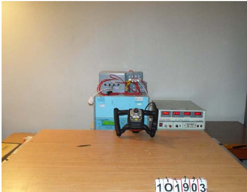
Figure 6 Harmonics & Flicker & Surge & DIPS test setup
