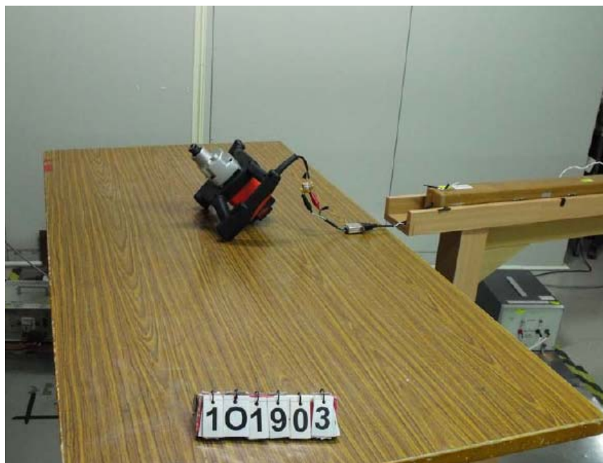
Figure 5 Disturbance power test setup
